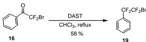
Scheme 9. Preparation of PhCF<sub>2</sub>CF<sub>2</sub>Br using DAST.
