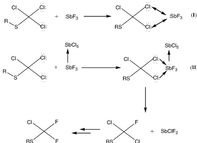
Scheme 3. Mechanistic suggestion of the role of  $\text{SbCl}_5$  in halogen-exchange reaction.
