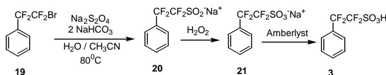
Scheme 10. Synthesis of PhCF<sub>2</sub>CF<sub>2</sub>SO<sub>3</sub>H.
