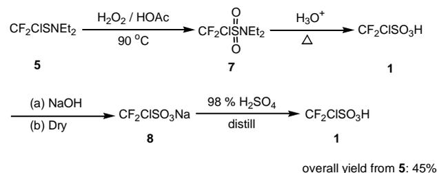
Scheme 4. Preparation of  $\text{CF}_2\text{ClSO}_3\text{H}$ .
