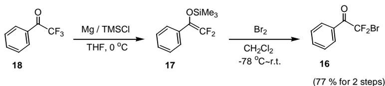
Scheme 8. Preparation of PhCOCF<sub>2</sub>Br.
