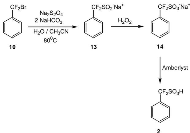
Scheme 6. Preparation of PhCF<sub>2</sub>SO<sub>3</sub>H.
